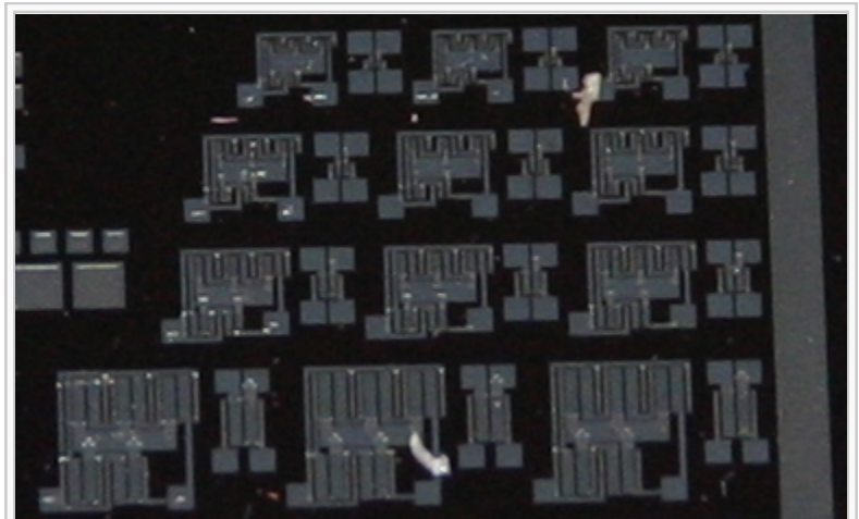
Ring oscillators fabricated on silicon using p-type MOSFETs.
