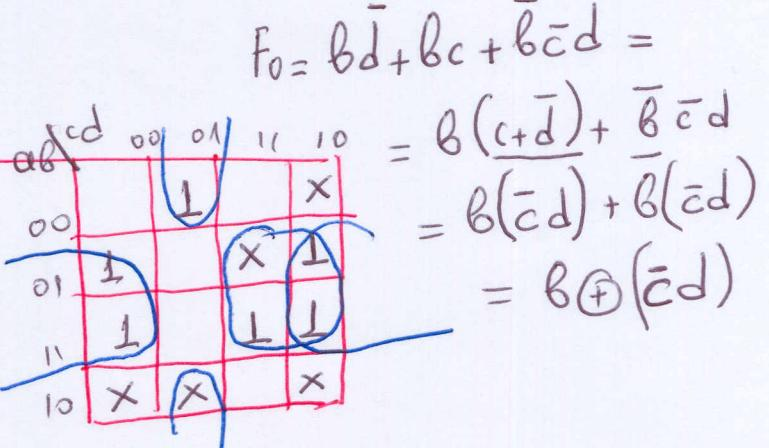
$$F_0 = \bar{B}\bar{D} + \bar{B}C + \bar{B}\bar{C}\bar{D} =$$
