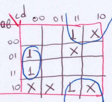
$$F_1 = \bar{B}C + \bar{C}\bar{D}B$$
